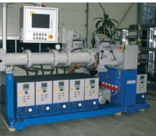
EEK 90.21 V for manufacturing of automobile profiles
