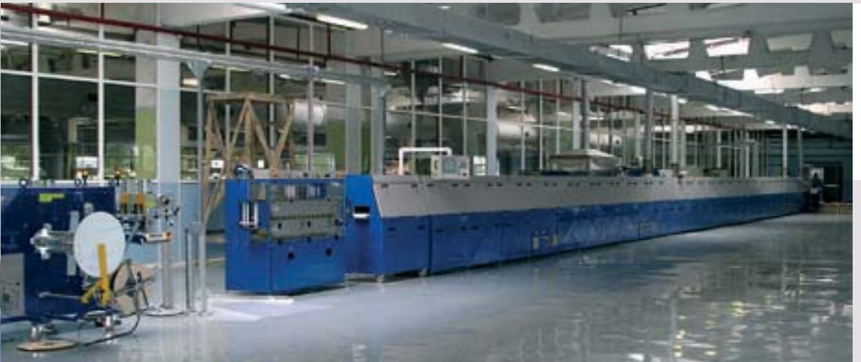
LCM 20 RS/EL Salt bath vulcanization line
