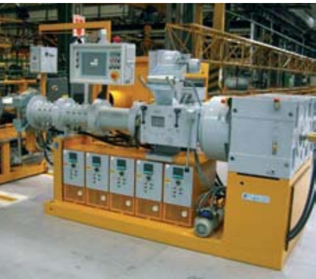
EEK 125.14 M for manufacturing of industry hoses
